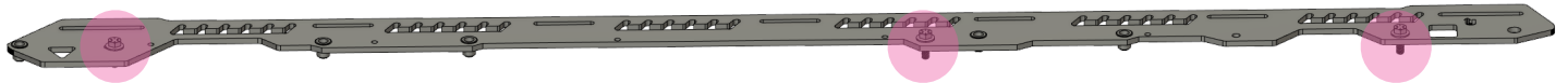
Figure 17 Subaru crossTREK Foot mount hole location(s). Driver Side (OUTER) shown. Front of rack shown on left side of illustration.
