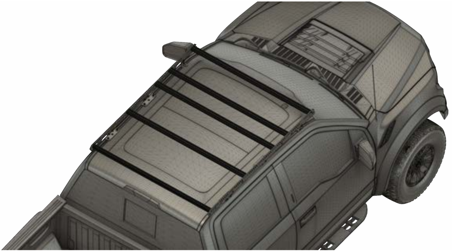
Figure 22 Rack to Roof
