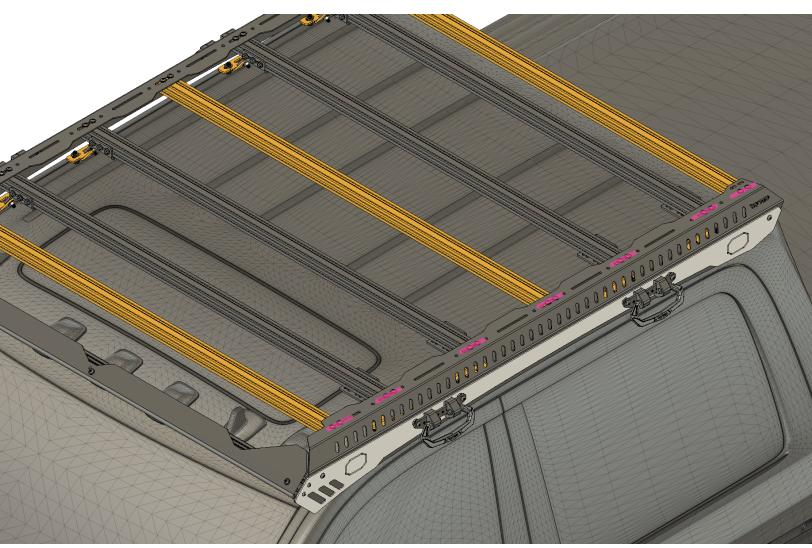
In this image the filled (cross bar) slots are shown in PINK. If you want to use any of these locations for your mounting brackets you would use the longer (smaller diameter) hardware to replace the ZULU factory hardware. Be sure to apply VC3 thread compound to the bolts.
