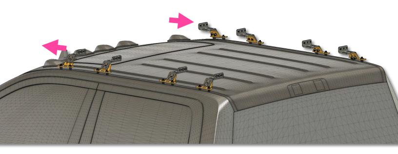
With all of the feet and cross bar clamps attached to the roof you are ready to install the first four (4) cross bars. A couple of notes before we get into that part....
