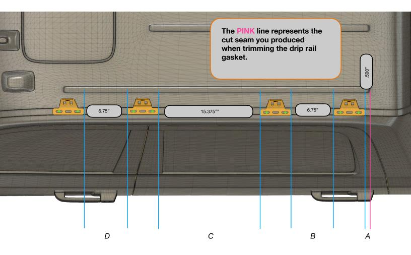
Use the feet as a template to mark the locations you will drill for roof rack mounting. Use the slots indicated in GREEN for each foot. Each location uses the same Z601 foot base.
