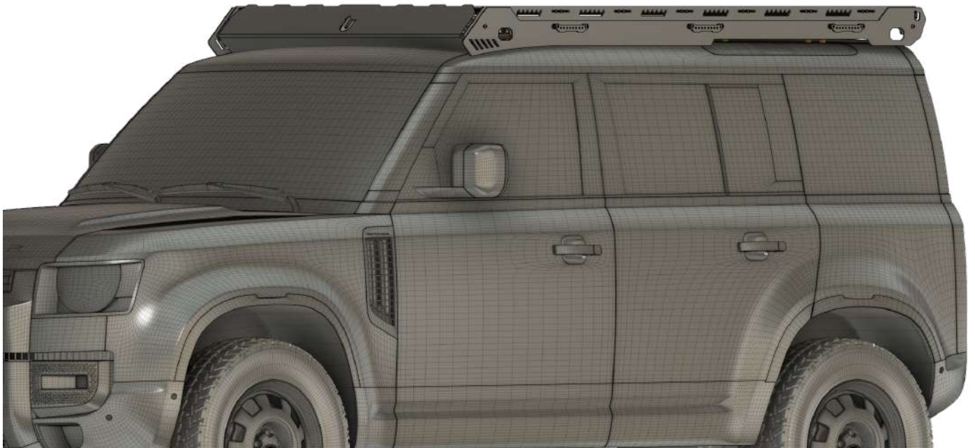
Figure 17 Installed Rover Rack Side Profile
