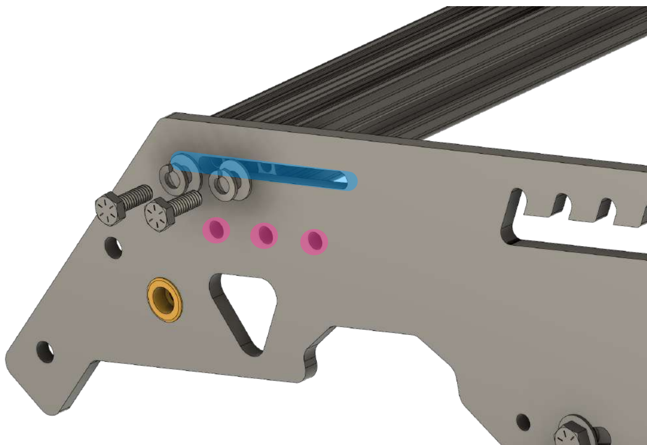
Figure 7 Driver Side 1075 Shown Front Load Bar Hardware Tools Required: 7/16" wrench
