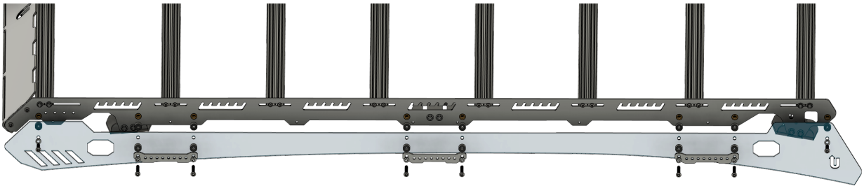
Figure 12 Driver Side Armor (1145) Shown Mating to Driver Side grooveTEK (1045) Front of Rack at LEFT of Image
