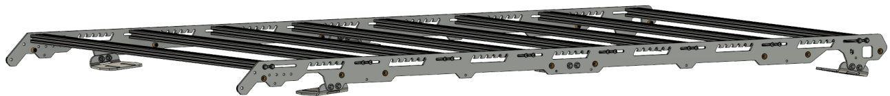
Figure 9 Progress Image All Feet and Load Bars Installed to grooveTEK. Driver Side Prominent / Front of Rack at LEFT of Image
