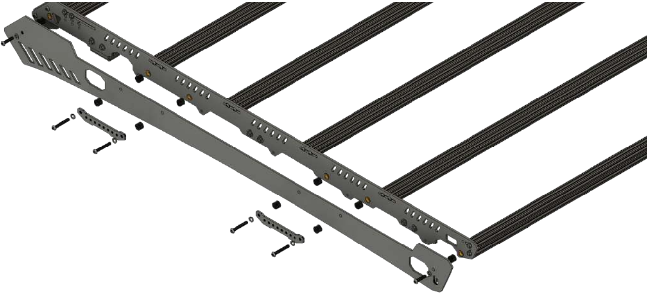
Figure 11A Driver Side (1175) Shown Armor to grooveTEK Hardware Exploded
