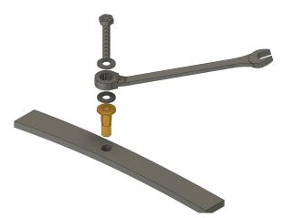
Assemble the included installation kit as indicated above. You'll need a small wrench (smaller than your washers, we use a 10mm), and an additional 10mm wrench or ratchet/socket to install the plusNUT
