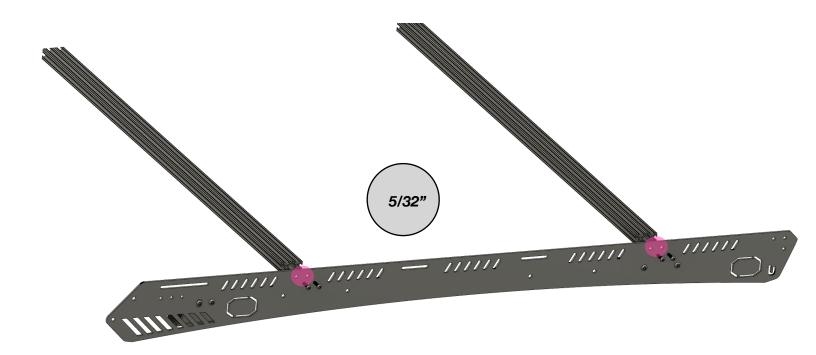
Start with the two positions located above in the Pink circles. These two positions are fixed (non-adjustable) and will make sure that your roof rack remains square (even from side to side).
