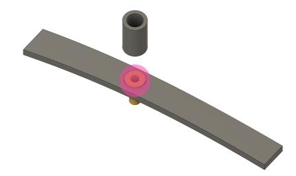
Before you lift the rack onto the truck again you've got to apply your sealant and place your spacers.
