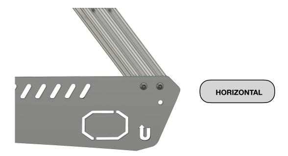
The remaining two cross bars are adjustable allowing you to shift them forward/backward in the slot. You can mount them at any position within the slot, just make sure they are even with each other on both sides of the rack.
