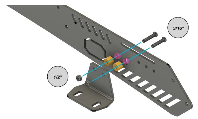
You are going to place those short aluminum spacers between the foot and the inside of the roof rack. This will give you the right alignment to your drip rails when you put the rack on the truck. Align the hardware to the hole and the slot highlighted in pink.
