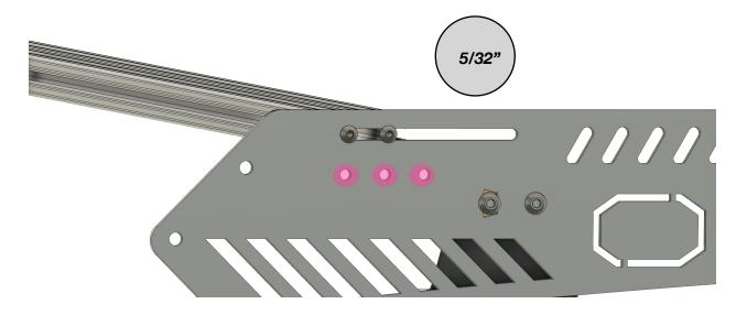
At the front of your rack you can install the load bar horizontally (as pictured) in the slot. You can also rotate the load bar vertically and use the slot for the upper bolt and any of the three holes shown in Pink for the lower bolt. The advantage of the vertical orientation is that the cross bar is more rigid turned on its side and we provide the two configurations to allow for options when mounting optional light bars into the front of your rack.
