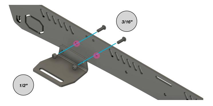
Line up your feet and install the hardware. Use the 3/16" Allen wrench and 1/2" wrench to tighten the feet.
