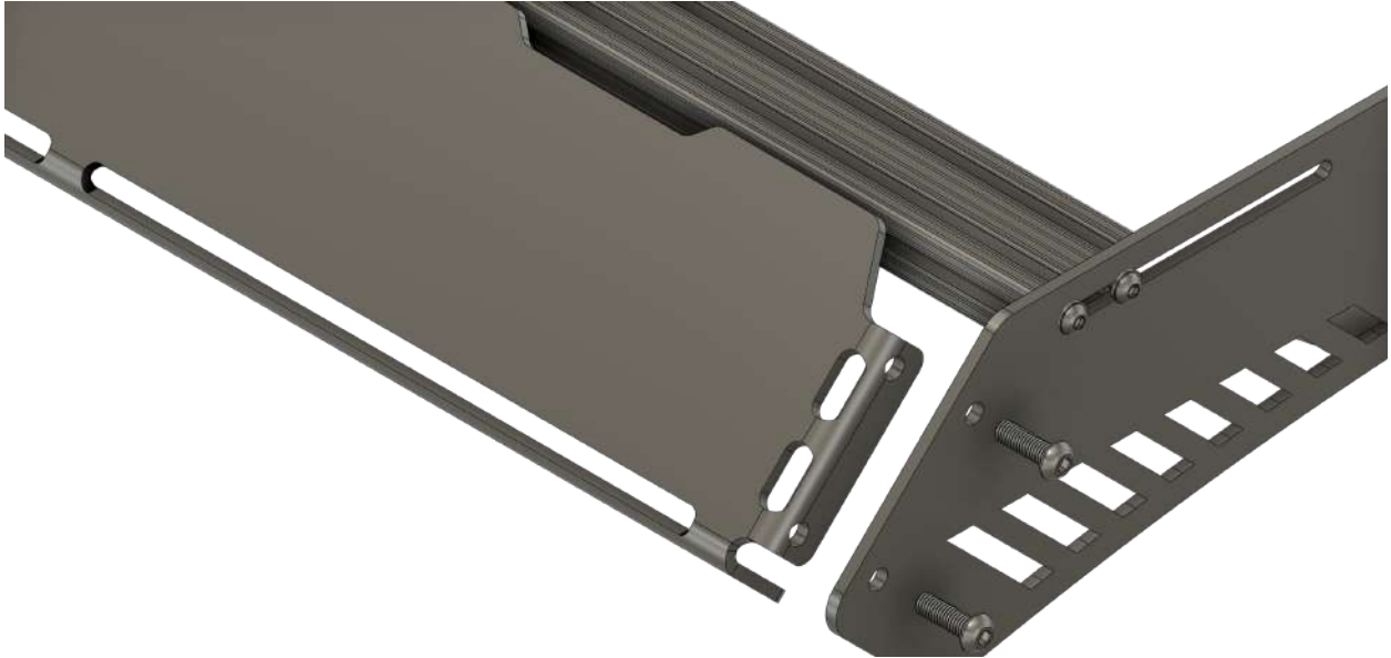
Figure 12 Fairing Installation Driver Side (2005.2) Shown
