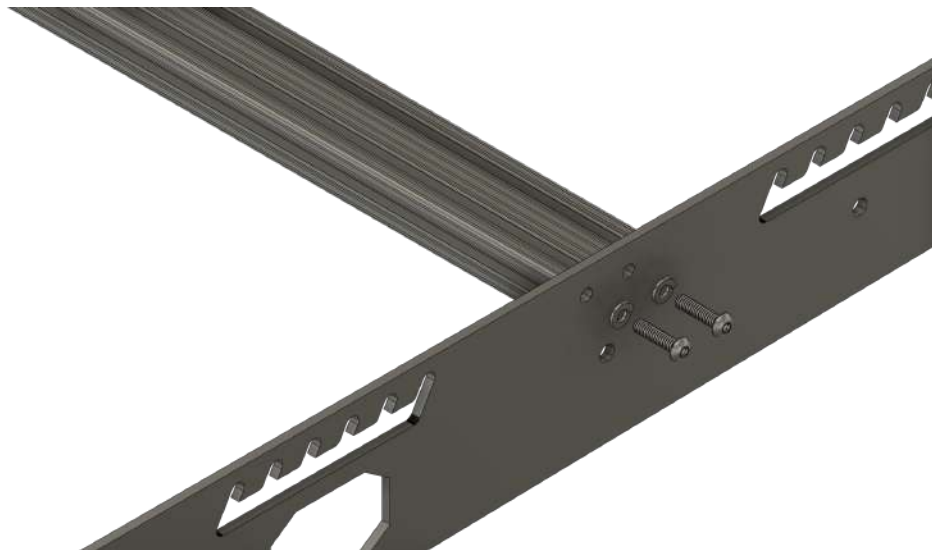
Figure 11 Fixed Position Load Bars 2/6 Driver Side (2005.2) Shown Slot Alignment
