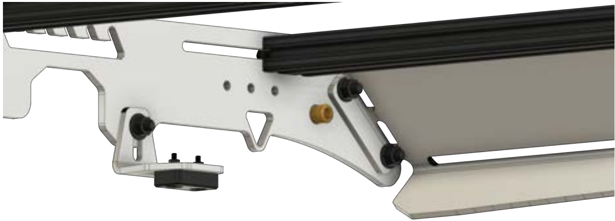
Figure 19 Fairing Hardware Completion-INNER SHOWN Driver Side grooveTEK (1011.3) Shown
