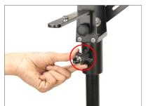
• Then loosen the rear section knob of the jib crane, as shown in the image.
