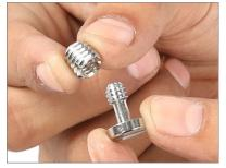
Insert 1/4" bolt into the provided thread of the bottom part of the extension camera plate, and from the top of the camera plate, insert it into the Conversion adapter bolt, by which the bolt size will be converted back from 1/4" to 3/8".
