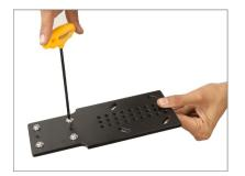
Match both the threads of the camera mounting head as well as the extension camera plate properly, and secure the screw with the help of a 4mm Allen Key.
