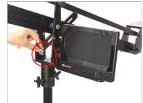
• Remove the jib crane from the jib stand.
