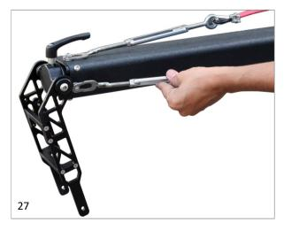
• Loosen side knob of Hub Mounting, slide it upwards to pull a small part out of it, for fixing cable later. Tighten the knob properly to secure it.
