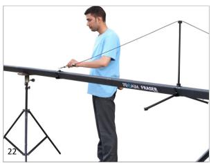
• Similarly, attach 18.5ft long (Red) cable from Section-1 to the end of Section-7, while aligning it with Cable Guide Top Rod.
