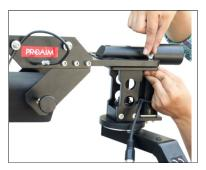
Attach one end of head cable to slot on head platform with the help of wire tensioner and another end with the cable already attached to central fork with wire tensioner as shown below.
