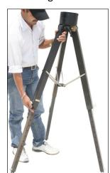
Match the holes of the bottom leg section with the upper leg section to secure the tripod stand with the Steel locking Pins and tighten the knobs.
