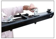
• Then attach 2 hooks to the hook that you attached (as per above image) with 1st, 3rd and 1 hook to 5th section.
