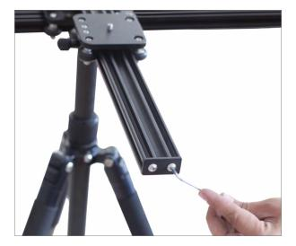
Tighten the knob to keep the camera plate stable at one place.
