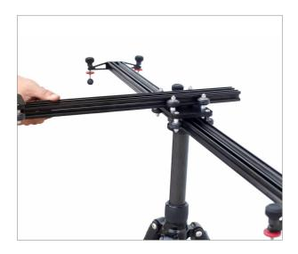
• Again attach the end plate with the top rail and tighten the allen bolts.
