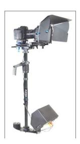
**Warning** If you do not have enough weight on the Base Platform the entire FLYCAM will flip upside down. Be prepared to catch it if this happens. You will need to add more weight to the base plate and retest until the FLYCAM remains right side up. The best way of adjusting the horizontal balance is to move the center of gravity of the Camera.
