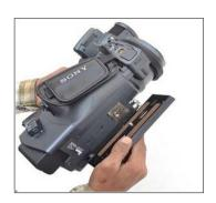
• Insert the camera plate into the base plate.
