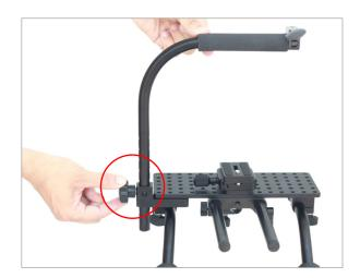
• Now take Shoulder Pad. Remove a bolt with the help of allen key to change the position of rod. Insert the bolt again and tighten with the help of allen key.
