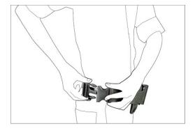
Insert the curved body support tube into waist belt and secure it with help of provided knob as shown. FLYCAM BODY POD 3
