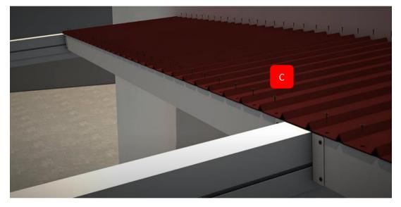
After the Interlayer profiles(15) are screwed into place, the cover sheets(C) are laid on the system. And they are screwed to the Interlayer profiles(15) at the front and to the wall connection steel profile at the back.
