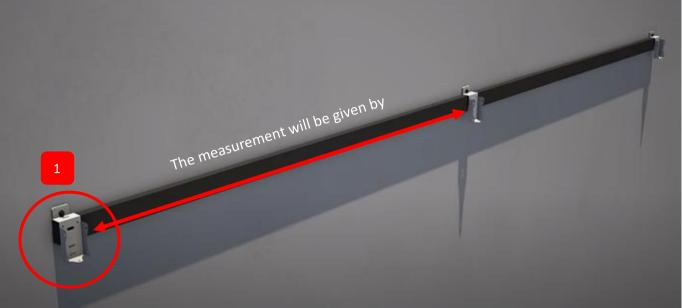
Firstly, the steel profile of the awning should be attached to the wall where the awning will be hung.
