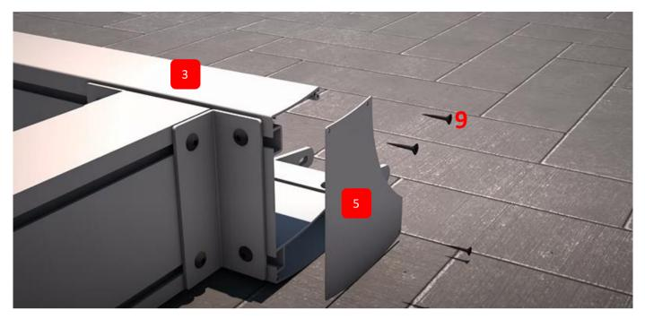
Gutter cover sheet(5) will be screwed to the Gutter Profile(3) with Star Head Screws(9).
