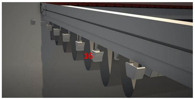
After all the cornices are in place, the Cornice caps(16) are installed. Electricity is supplied to the motor and it is checked whether the fabric is tight. Then check whether the system is working properly. Accordingly, the Gutter-Rail connector(4) is tightened and the rails are
