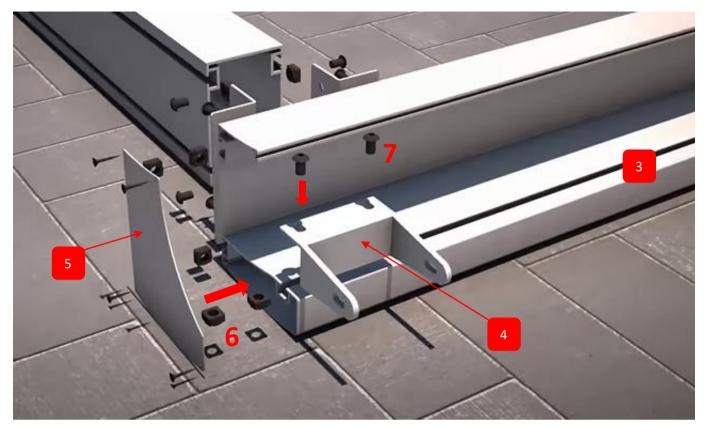
The Gutter-Rail connector(4) will be screwed onto the Gutter Profile(3) with Square Nut (6) and allen head screw (7) but should not be tightened too much. The gutter-rail connector(4) should have some movement.
