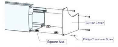
Gutter covers are mounted to the gutter profiles.
