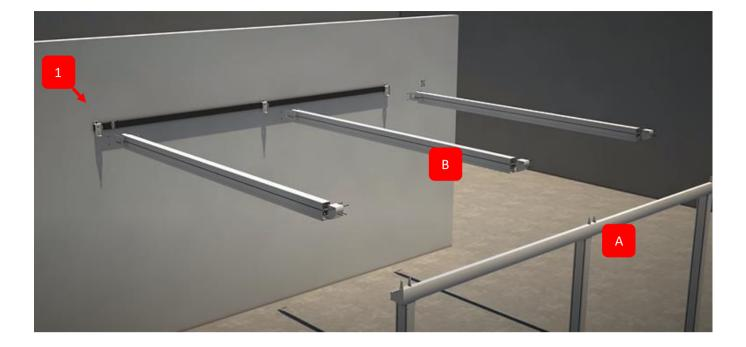
The rails(B) will be assembled one by one to the U-brackets(1) and Frame(A).
