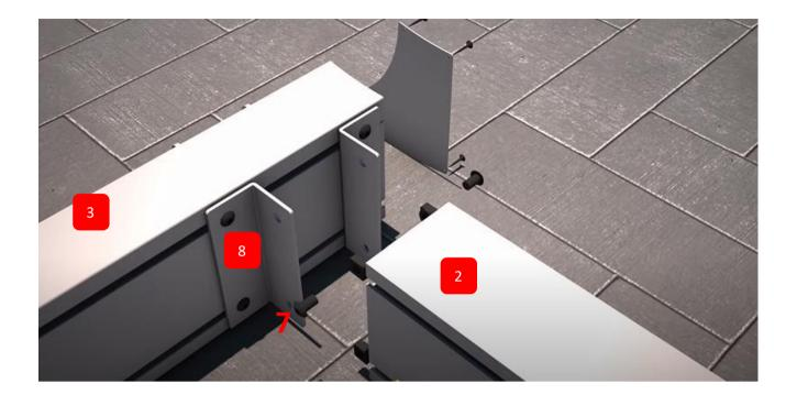
After L-Connection parts(8) are screwed to Gutter Profile(3), The Pole Profile(2) will be assembled to the L-Connection Parts(8) L-Connection Parts(8).
