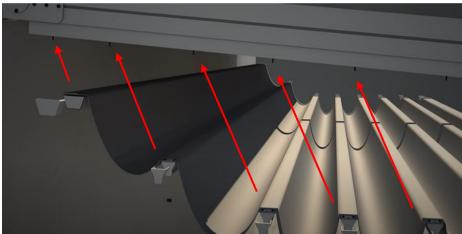
The pvc polyester fabric(D) with the cornices is attached to the casters placed on the rail profiles in such a way that it fits into the holes in the cornices. Each caster is placed in a cornice hole. After the fabric cornice is attached to the casters it is tightened with a nut and its cover is attached. 16
