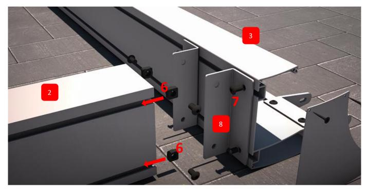
For the connection of pole profile(2) and Gutter Profile(3) , L-Connection Part(8) must be screwed under the Gutter Profile(3) with allen head screw (7) 7
