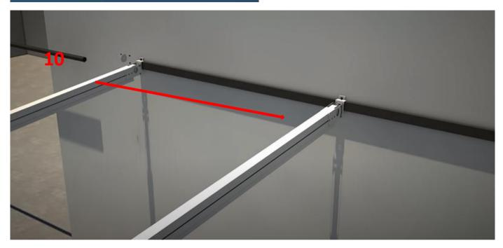
The Motor Pipe Profile(10) is inserted into place by passing it through all the rails
