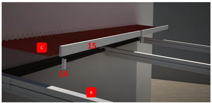
In order for the cover sheets(C) to be mounted, the Interlayer Profiles(15) must be placed between the Rail Profiles(B). The Connection plate(14) that will hold this profile must be screwed to the rails(B).
