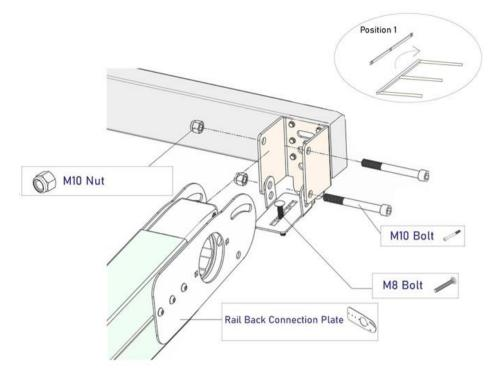
3.Collecting Water Gutter Profile Parts and Connecting to the Pole Profiles
