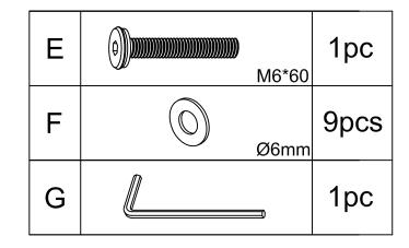
Note: first screw all bolts in by hand, before tightening.
