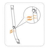
2 Align the flange with the holes on the steering wheel and tighten it with four M5 screws with the 4 mm hex wrench.
