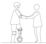
2 Lightly place one foot on the foot mat, while keeping your other foot on the ground holding your weight. Do not press the steering bar with your leg.
