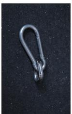
5. Step five we will be using the second carabiner and connecting the pully loop attachment together. For this we will slide the open side of the attachment onto the carabiner. This makes it possible for the pulley system to perform its task.
