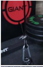
10. For step ten we will be applying the Pulley Lock Attachment that locks both sides of the cable together.
