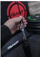
9. For the bottom of the cable we will be putting it around the loop attachment. With your fingers squeeze the rope together.
