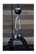
Attach the Carabiner to the cable that is suspended in the air. From there you are able to attach the rope. After this step you are ready to start using your new pulley system! Just add some weight!
