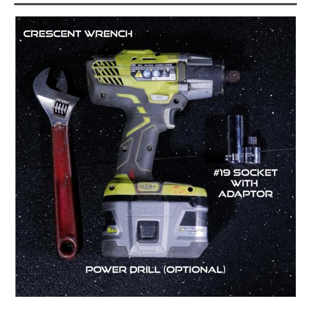
For this project we will need the following a **Crescent Wrench** and or **Socket Wrench**. If available a **Power Drill** which will speed up the process of building. If a power drill is being used, use a #19 Socket as it matches the bolts that we are using!
