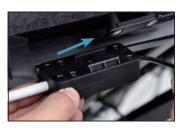
**e.** Connect The Wand to the Control Box Cable via the 3-pin connector.
