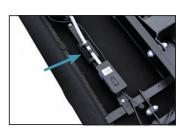
Insert the Power Cord into the Power Supply.
