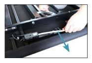
**d.** After removing the offline voice box, when installing on the other side, slide the wand device onto the mounting bracket until you feel it click into place.
