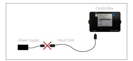
Connect the end of the Battery Backup Strap to the input cord that is attached to the control box.
