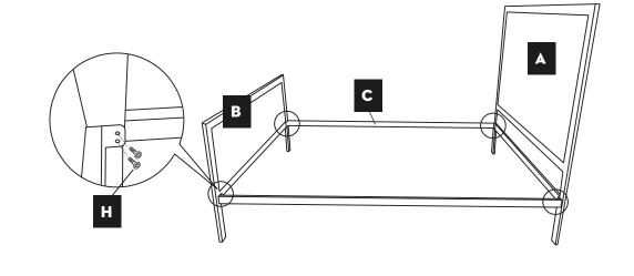
Connect center support bar (D) to the headboard (A) and footboard (B) using 15mm bolts (H) and the ratchet tool (J).
