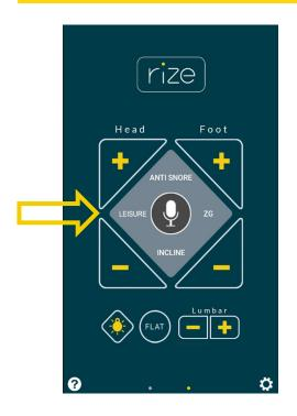
Tap the preset button you want to activate. The preset buttons are ANTI SNORE, LEISURE, ZG (Zero Gravity), INCLINE, and FLAT.
