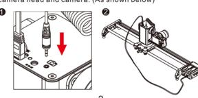
6 ) Install the battery on the slider and check the signal cable or shutter cable connecting correctly or not. (As shown below)
