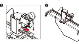
${\bf 5}$  ) Use the shutter cable to connect the motorized camera head and camera. (As shown below)
