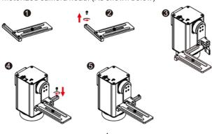
2) Mounting the motorized camera head on the slider. (As shown below)
