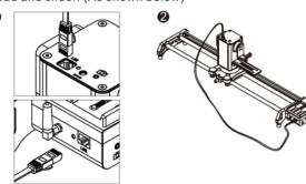
4) Mounting the camera on the slider. (As shown below)
