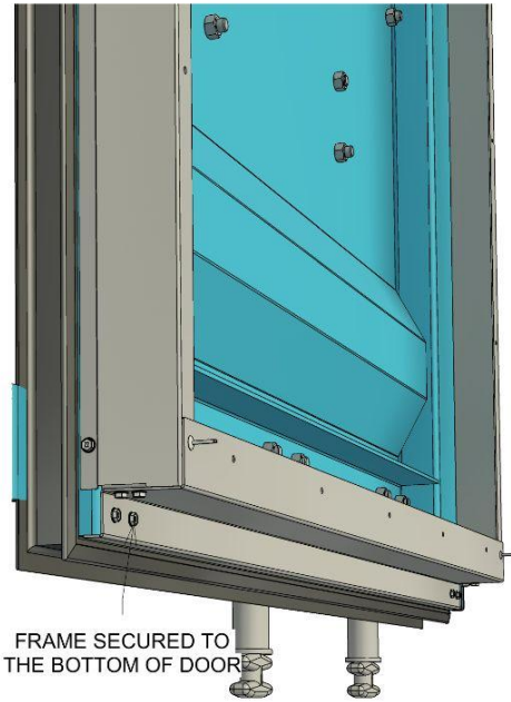
Figure 6 - Flashing Kit Installation Container Door Bottom
