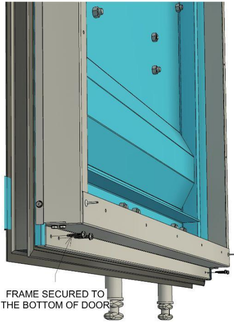
Figure 5 - Bottom sides connected to footer
