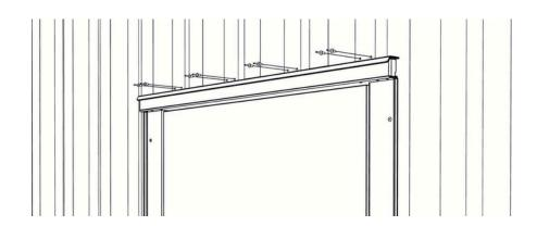
• From the outside of the container, rivet the rain drip to the container wall with a rivet gun using the holes from Step 8.
