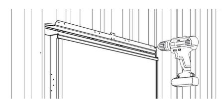
• Pre-drill the rain drip fastener holes from the interior of the container.
