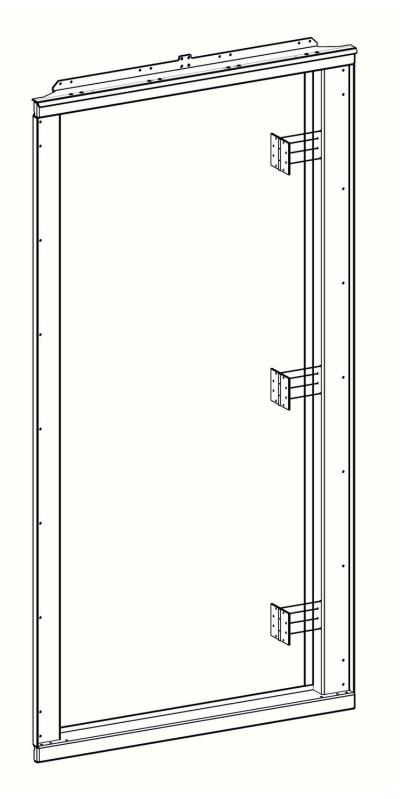
Mount hinges to the frame as shown, using the screws provided in the hardware package.
