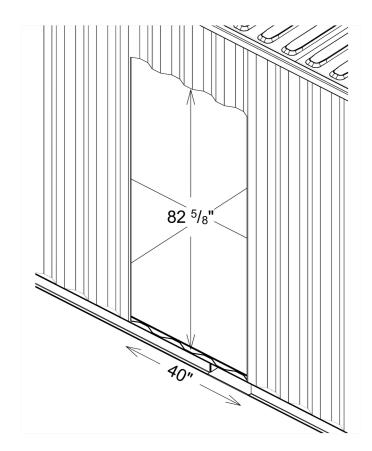
\*Cut above the bottom weld, not flush to the container floor
