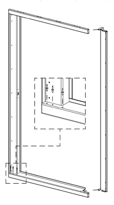
Fasten frame sides to header and footer using a rivet gun and the rivets provided.
