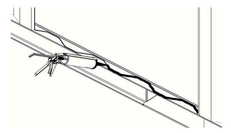
• Apply caulking around the bottom of the cut out where the door footer will sit.
