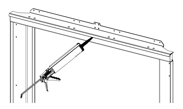
Apply silicone to the underside of the rain drip using a caulking gun to cover all exposed rivets.
