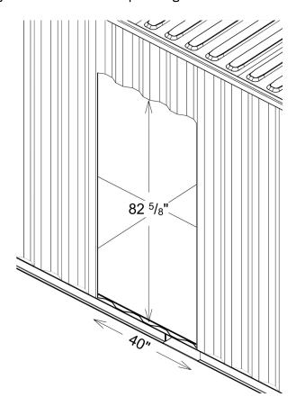
\*Cut above the bottom weld, not flush to the container floor
