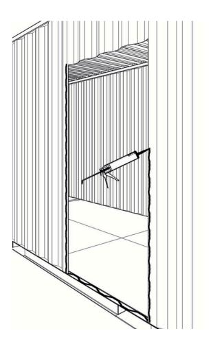
• Apply caulking to the exterior of the container, where the door sides will sit.
