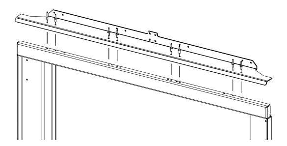
• Rivet the rain drip to the frame header.
