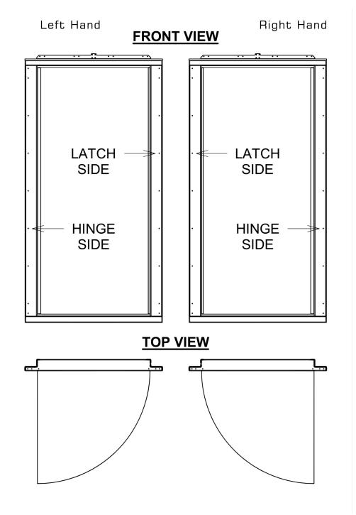
• Determine if you will be installing on the side wall or end wall, with a left or right hinge side. By turning the frame over you can determine the swing of the door. 2
