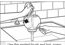
Use the angled brush and hot, soapy water to finish cleaning the brew unit; then, rinse with clean water. Allow to air dry with the lid removed, or dry with a soft towel.
