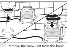
unit stand and place it on the carafe with handle to the right or left of the carafe handle. Turn the brew unit handle until it aligns with the carafe handle and locks into place.
