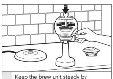
grasping the brew unit handle, and use the coffee filter handle to place the coffee filter into the bottom of the brew unit. Turn the coffee filter handle clockwise until the coffee filter locks into place.
