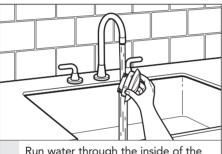
Run water through the inside of the lid after every use. Prop the lid on its 7 side to allow it to fully air dry.
