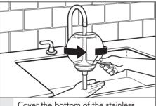
Cover the bottom of the stainless steel siphon tube with the palm of your hand. Fill the brew unit with hot tap water, moving it in a circular motion to rinse away remaining coffee grounds.
