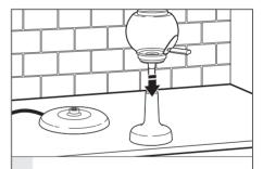
Place the brew unit stand on a flat. sturdy surface. Insert the stainless steel siphon tube into the brew unit stand.
