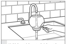
Hold the stainless steel siphon tube above a sink and remove the palm 4 of your hand to empty the water and coffee grounds from the brew unit. Repeat steps 3 and 4 as needed.
