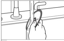
After brewing, untie the drawstrings, remove the cloth filter from the stainless steel filter disc, and carefully rinse in running tap water to remove all residue.
