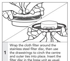
**NOTE:** Make sure to tie the drawstrings securely, but leave enough slack to allow for removal when you are finished brewing.
