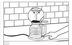
Press down on the ON/OFF switch to begin the brewing cycle. The LED indicator will glow and the water will begin to heat.
