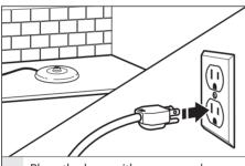
Place the base with power cord on a flat, sturdy surface and plug it into a grounded outlet. If desired, wrap excess cord around the cord holder on the bottom of the base.
