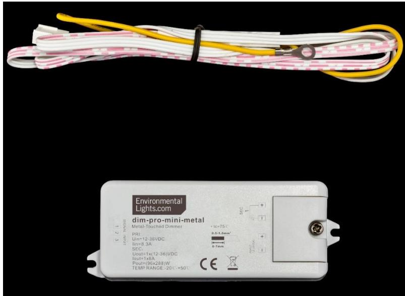
The Mini Touch Conductive Dimmer with Receiver turns a conductive metal surface into a touch control for single color LED lights. The sensor tip can be easily secured to any metal surface up to a meter away from the dimmer housing. That surface or object will serve as the on/off switch and dimmer control for up to 8-amperes of LED lighting. Tap anywhere on the conductive surface to cycle through 4 levels of brightness and to turn the lights off.
