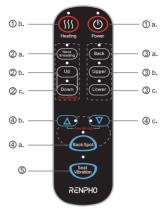
1. Press the "Power" Button to turn on the massager; the indicator light will turn red to show that the massager is on. The Neck Kneading and Full Back Massage functions are on by default. Seat Vibration function and the Heating function of neck and back are off. The indicators on the remote will remain in the "on" status accordingly. 2. Activate the functions you need.
