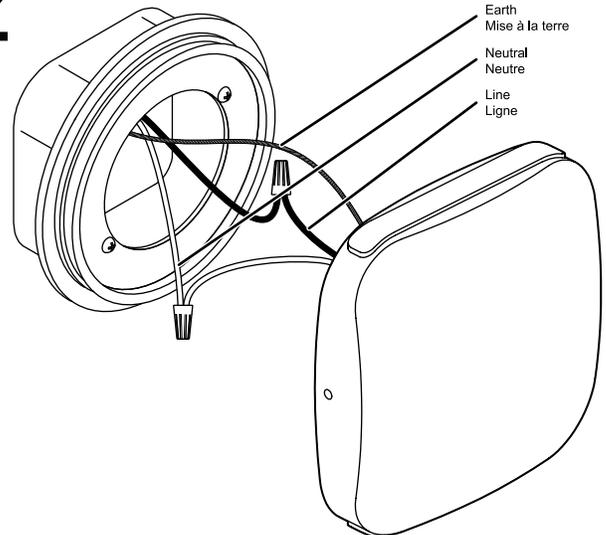
Make connections in the compartment: use the included wire connectors to match the white wire from the line feed with the white wire from the fixture and to match the black wire from the line feed with the black wire from the fixture. Then, match the copper wire from the fixture to the ground screw on the round plate.
