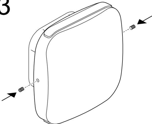
Pull all the wiring inside of the electrical box and screw the fixture on the mounting bracket using the 2 set screws.
