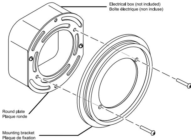
Install the round plate on the electrical box, then screw the mounting bracket on the round plate.
