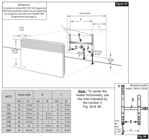
To install the heater at 10 cm (4 in) from the floor (recommended height by CONVECTAIR) follow these steps:
