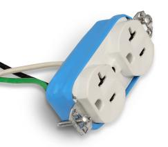
The **NEW ArmourBand™ Insulating Wrap** insulates and protects devices while providing a quick, clean, reusable solution to the traditional tape application. It fits most receptacles while offering a repositizonable wrap with a non-slip finish, allowing for excellent grip that leaves no residue behind.
