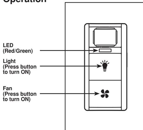
**NOTE:** When the RED and GREEN LEDs are on at the same time, the light will appear as an AMBER color.
