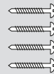
4 to 6 No. 6 to No. 10 round-head wood screws and suitable brackets to secure the fan heater (4.3 kg or 9.4 lb) to the type of wall
