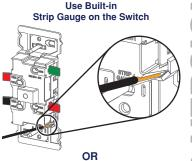
**Use Strip Gauge** as shown below (measure bare wire here)
