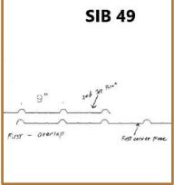
**2.** The 2nd roof panel must overlap the first piece by 1/2 a sheet. Finish screwing first panel down going through panel one and panel two.
