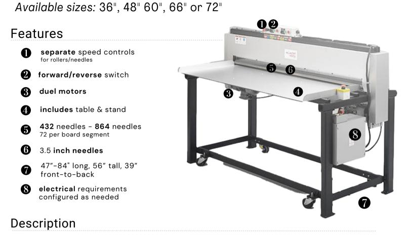
The **FELTLOOM**® **Pro Series** features *two* motors that power the needleboard & rollers, allowing the operator to adjust the speed of each independently.
