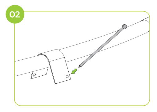
Insert the **Peg (2)** through the outer hole on the **Bracket (1)** at a 45 degree angle. Push or hammer the **Peg (2)** into the ground.
