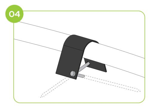
Repeat the steps, placing the ANCHORKIT  $^{\text{\tiny{M}}}$  assemblies on opposite sides of the trampoline.
