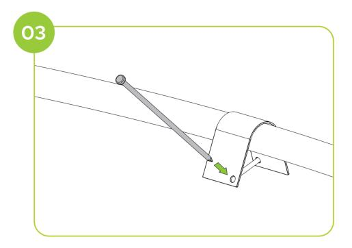
Insert the **Peg (2)** through the inner hole on the **Bracket (1)** at a 45 degree angle. Push or hammer the **Peg (2)** into the ground.
