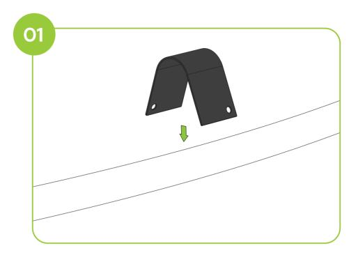
Place the **Bracket (1)** in the center of the lower rail between two legs. Ensuring either side of the **Bracket (1)** touches the ground.
