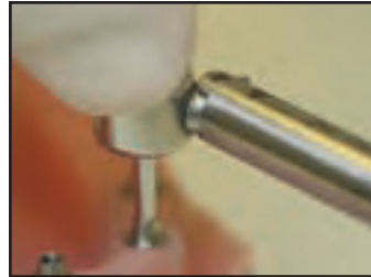
Torque Applied (Wrench head in release/broken position)
