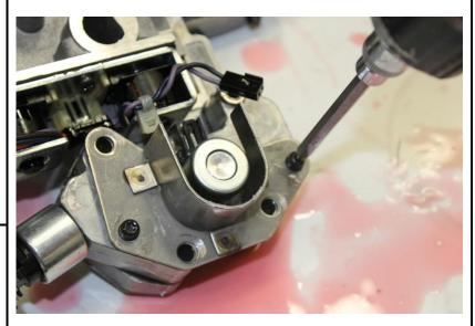
Reconnect governor solenoid connector if it was disconnected during the install.
