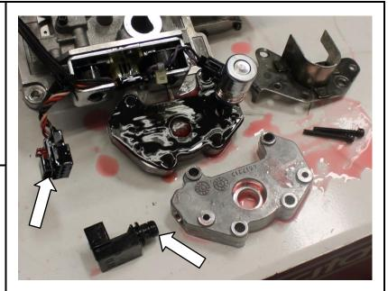
Lubricate the O-ring on the new sensor with ATF and insert into the governor housing.
