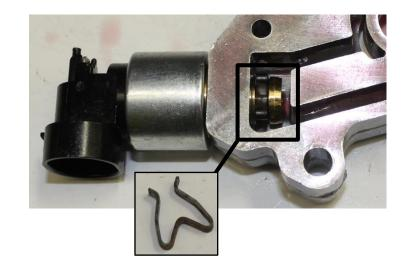
The metal retainer bracket will not fit around the new sensor, so the bracket can either be notched with a cutting wheel or the two tangs may be bent out of the way.
