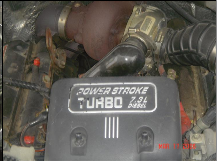
Hose not installed
