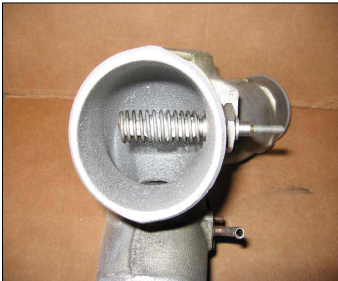
Intake with Heater Installed
