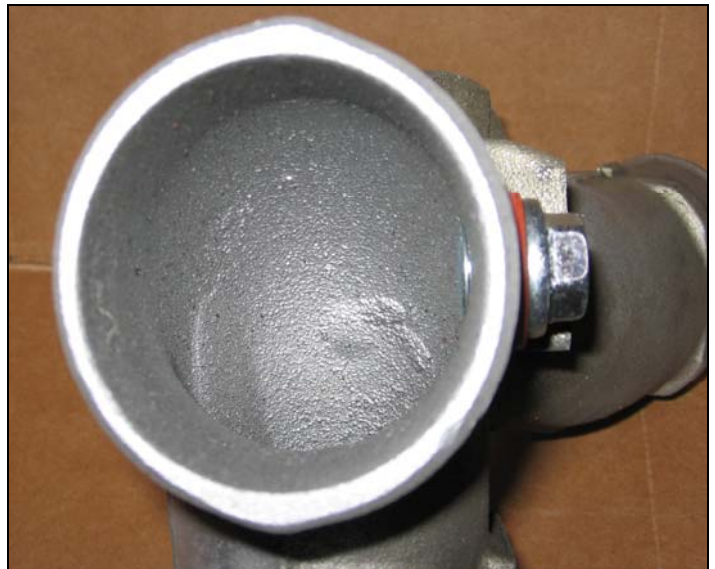
Intake with Heater removed
