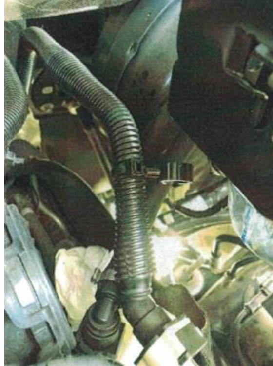
Figure 11: Proper hose clearance
