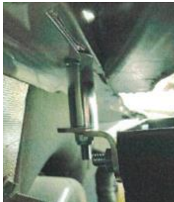
Figure 7: Bracket installed with spacer
