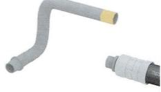
**Step 4.** With the steel lines clean and deburred, put a small amount of oil on the end of the line before sliding the repair line fitting over the steel line. Check fittings for proper assembly. With fitting loose, slide the fitting over the tube until it bottoms out. Tighten the nut on the repair line fitting until you can no longer turn the steel line in the fitting. After lining up the orientation of the line as noted in step 2, you can tighten the other side.
