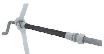
**Step 5.** Be sure to install cooler lines back into all existing factory clamps to avoid rubbing on suspension or other components. Check for leaks.
