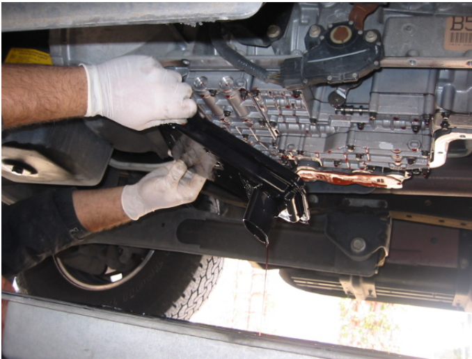
(Figure 3) Transmission Filter Removal
