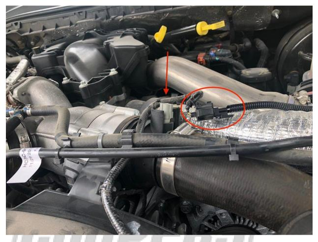
**TIP:** Some of the newer models will have the sensor located right on the top of the black intake hose instead of underneath
