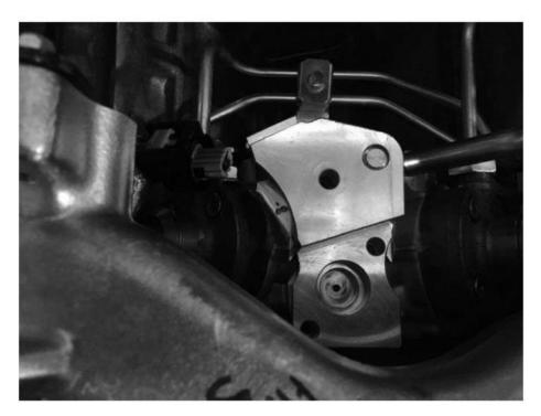
Install metering unit and tighten all fasteners.
