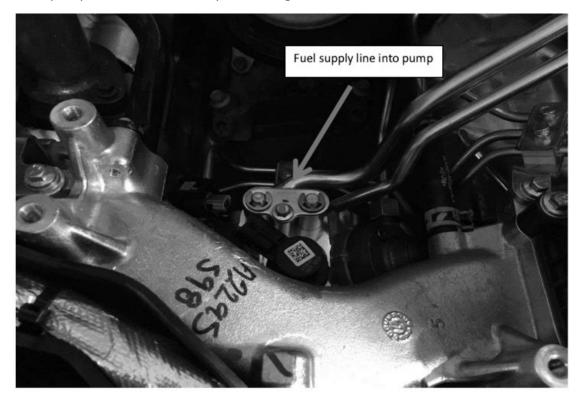
Removal of the fuel filter and fuel filter base housing is required to gain clearance to remove the upper plastic air manifold. Remove the hard plastic line from the filter to the fuel supply steel line that goes to the high pressure pump. The supply line to the pump is on the passenger side of the pump. See pic above.
