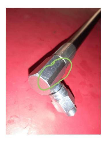
**Note Before Install:** It is highly recommended that you do the following modification before install. Grind a small section of the circled area of the swivel fitting as shown in the picture above. The approximate cut is about 1/8" inch.
