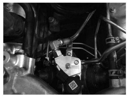
Note: This 2 wire braided hydraulic line must not touch any component as it is fit into the valley and run out.
